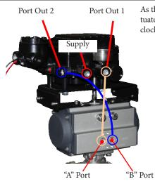
As the pressure increases, actuator stem rotates counterclockwise.
