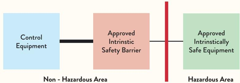
There is a fundamental difference between intrinsic safety and the other equipment application techniques. None of the others aims at preventing release of energy at a dangerous level.
