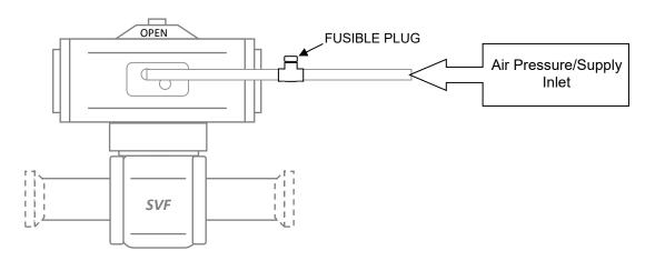
Fusible plug devices are limited in applications where the service pressure does not exceed 500 psig (3,440 kPa). The fusible plug devices are available in brass or stainless steel construction and are available in design temperatures listed in the table below.
