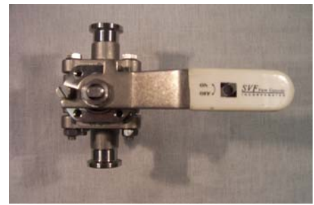
VALVE IS CLOSED
