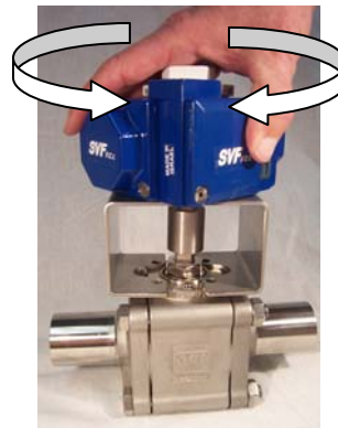
Loosened actuator may serve as a manual operating device to position a valve for maintenance.
