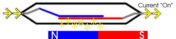
2. Switch closes when magnet is near
